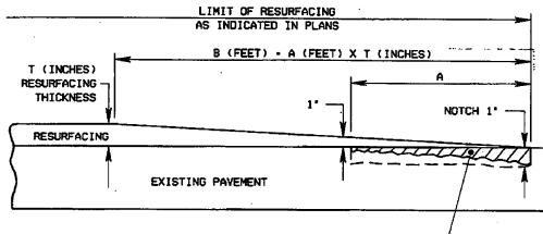
WHEEL RUTS BEYOND THE HEEL-IN NOTCH ARE TO BE FILLED AND TRANSITIONED TO MEET FIELD CONDITIONS.
